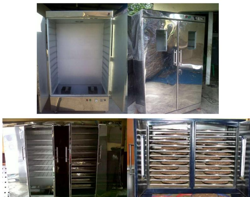
**Gambar 1. Ruang Dan Rak Pengering Cabinet Dryer System Multi Energy.**
